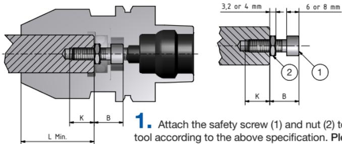
**1.** Attach the safety screw (1) and nut (2) to the shank tool according to the above specification. **Please Note**, in order to get correct balancing and performance, it is very important to keep the specified measurements.
