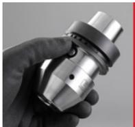
**3.** Compress the safety mechanism with your finger.
