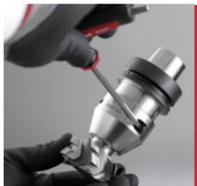
**5.** Remove your finger from the safety mechanism. Tighten the pressurizing screw until it stops, **max 6 Nm!** Any higher tightening torque will not increase the fastening force. Make sure to keep the tool completely inserted into the chuck as you pressurize the unit.
