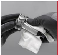
**2.** The tool and the G3 chuck must be thoroughly cleaned, removing all traces of grease and other impurities.
