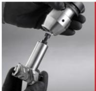
**4.** Place the shank tool in the chuck, making sure that the tool is completely inserted and the safety mechanism is still compressed.
