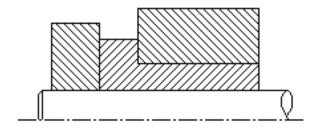
By varying the tightening torque the slip torque will change. In this way ETP-TECHNO can be used as a torque limiter, if the slippage only occurs very shortly and only for a part of a revolution.
