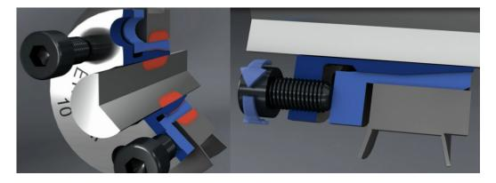
The screws, at least one, need to be dismantled completely and moved to the threaded bore in the flange. When tightening, the screw will push the two sleeves apart.
