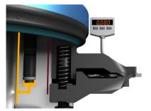
3 Pressurize and clamp the tool by using an allen T-wrench at the red (A) position on the adjustable unit. Turn the Allen key wrench until the system is fully pressurized and the pressurizing screw reach a firm stop (5 Nm).
