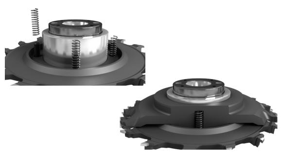
Release the pressure on the outer system, indicated (A), on the hydro sleeve. Place the four CUBIT springs on the bolts and slide the adjustable tool part onto the hydro sleeve. Make sure that the tool is positioned in such a way that the holes on the under face matches the location of bolts and springs. Pay special attention to the springs are inserted into the holes in the adjustable tool part.
