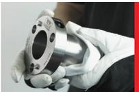
**1.** The tool and the hydro sleeve must be thoroughly cleaned, removing all traces of grease and other impurities.
