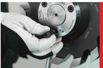
**3.** Make sure the holes in the flange match the threaded holes in the tool.
