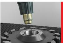
**2.** If the tolerances of the tool bore and the ETP HYDRO GRIP allow a light press fit, heat the cutting tool until the ETP HYDRO-GRIP easily fits into the tool (approx. 70°C).
