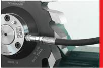
Connect the high pressure pump and increase the pressure to 400-450bar (5800-6500 psi).
