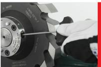
**4.** Mount the whole unit onto the grinding machine spindle. Tighten the pressurizing release nipple, maximum 3 Nm-27lbf.in.
