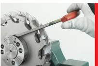
**3.** Mount the whole unit onto the grinding machine spindle. Pressurize the sleeve by turning the Allen T-wrench a few turns to approx. 2 Nm (1,5 ft lbs) until you feel the tools are centered.
