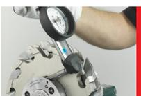
**5.** Tighten the pressurizing screw until it stops, max 10 Nm (7.4 lbs). Any higher tightening force will not increase the fastening force.
