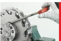
**7.** Release the pressurizing screw with an Allen T-wrench. Remove the tool unit from the grinding machine and it is now ready to be installed on the machine.
