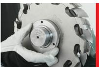
**2.** Mount the tool/s and spacers onto the hydro sleeve, tighten the locking nut lightly in order to keep the tools closed to each other.
