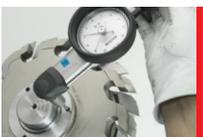
**4.** Tighten the screws (hexagon socket head, 3mm) uniformly in the locking nut. Required torque 3-4 Nm (26-35 lbf.in). Thin tools or longer sleeves (+ 120mm, 4 3/4") 6-8Nm (53-70 lbf.in)
