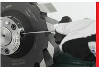
**3.** Mount the whole unit onto the grinding machine spindle. Tighten the pressurizing release nipple, maximum 3 Nm-27lbf.in.
