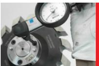
**5.** Tighten the locking screws (M8) through the flange to a min. 8 Nm (6lbs).
