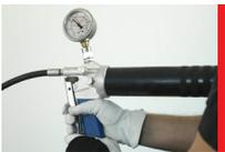
**4.** Connect the high pressure pump and increase pressure in 50 bar (700 psi) increments until all the tools are centered.
