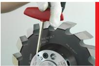
**3.** Mount the whole unit onto the grinding machine spindle. Pressurize the sleeve by turn the Allen T-wrench a few turns to approx. 2 Nm (1,5 ft lbs) until you feel the tools are centered.
