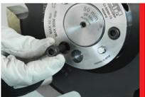
**2.** Mount the tools and spacers onto the hydro sleeve. Insert locking screws through the flange of the sleeve and tighten the screws finger tight.
