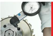
**4.** Tighten the locking screws (M8) through the flange to a min. 8 Nm (6lbs).
